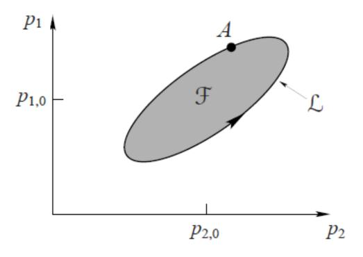
Figure 4.2: During one period the point A(t) with coordinates  $(p_1(t), p_2(t))$  follows a trajectory  $\mathcal{L}$ .  $\mathcal{F}$  stands for a surface area. The arrow indicates a movement direction for  $\varphi > 0$ .
