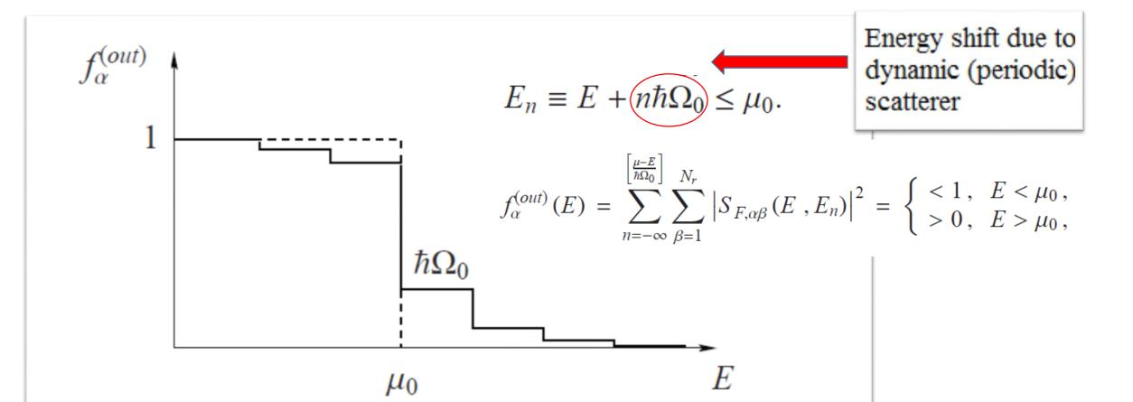
Figure 4.1: The non-equilibrium distribution function,  $f_{\alpha}^{(out)}(E)$ , for scattered electrons at zero temperature is shown schematically. The step width is  $\hbar\Omega_0$ . The zero-temperature Fermi function is shown by dashed line.
